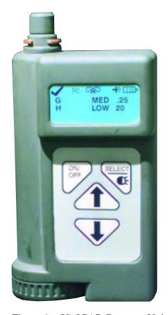
Figure 1. (U) JCAD Detector Unit
