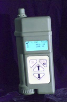
(U) The low level detection requirements are accomplished with the use of a preconcentrator (PC). Figure 2 shows the detector unit with the PC attached. The PC is a Figure 2: (U) JCAD Detector Unit with Pre-Concentrator Attached
