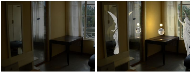
Figure 8: Our method allows for light source insertion and easy material reassignment. Here, a glowing ball is inserted above a synthetic glass sphere, casting a caustic on the table. The mirror has been marked as reflective, allowing synthetic objects to realistically interact with the scene.
